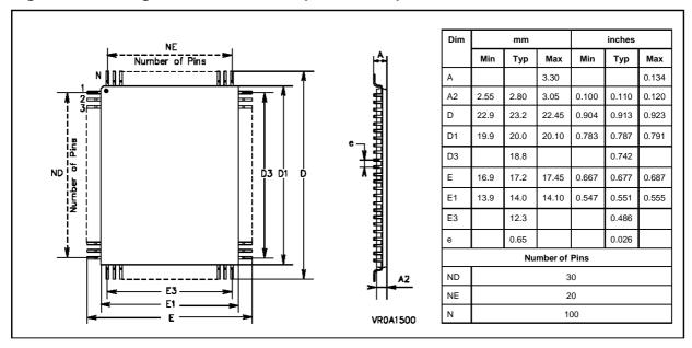
Figure 24. Package Outline TQFP100 (14 x 14 mm)
