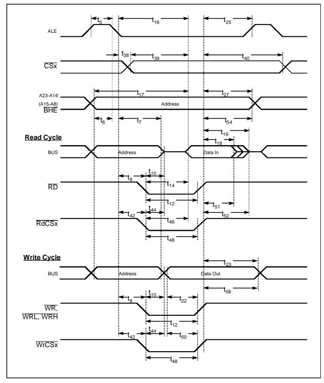
Figure 12. External Memory Cycle: Multiplexed Bus, With Read/Write Delay, Normal ALE
