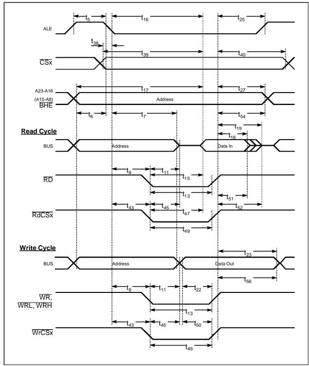
Figure 15. External Memory Cycle: Multiplexed Bus, No Read/Write Delay, Extended ALE
