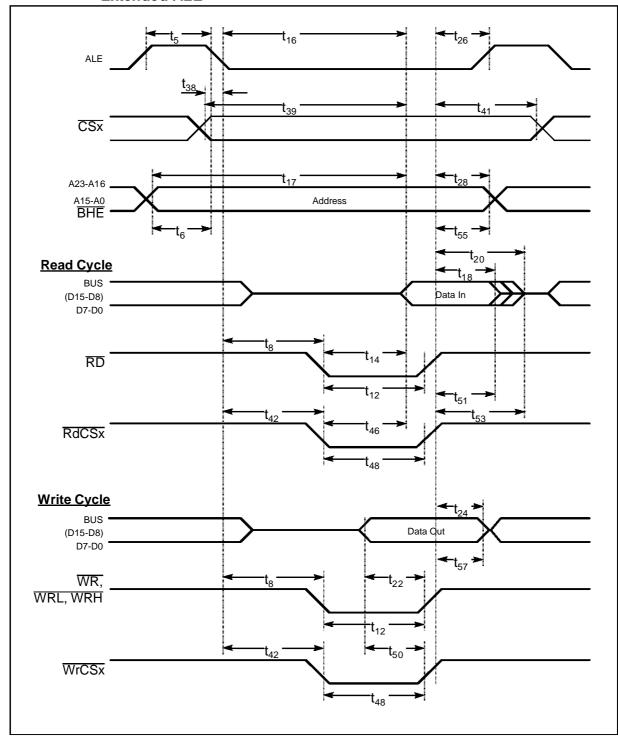
Figure 17. External Memory Cycle: Demultiplexed Bus, With Read/Write Delay, Extended ALE
