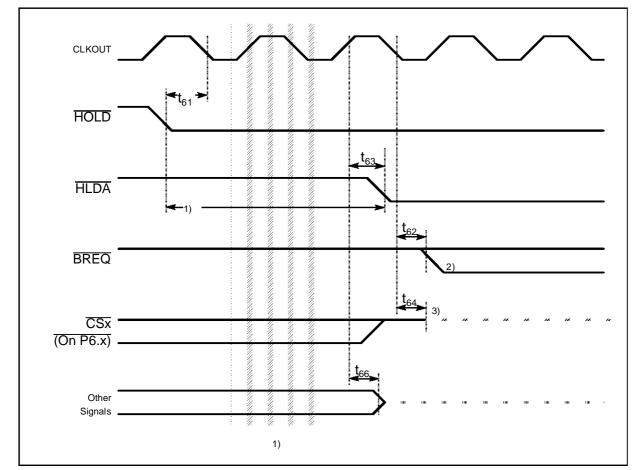
Figure 21. External Bus Arbitration, Releasing the Bus
