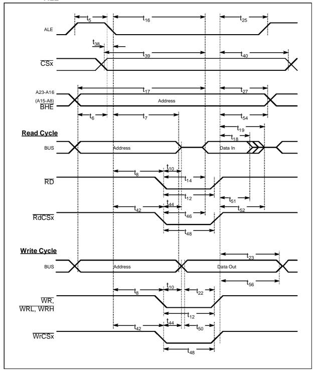
Figure 13. External Memory Cycle: Multiplexed Bus, With Read/Write Delay, Extended ALE
