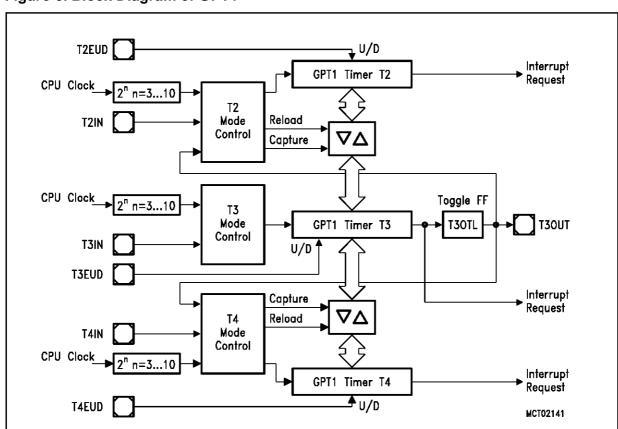
Figure 6. Block Diagram of GPT1
