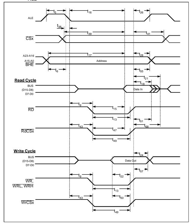
Figure 19. External Memory Cycle: Demultiplexed Bus, No Read/Write Delay, Extended ALE
