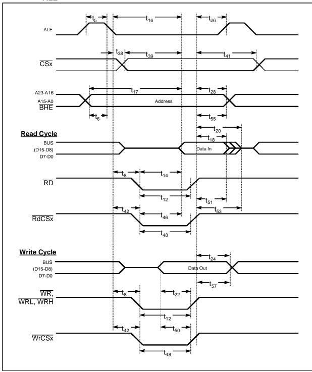
Figure 16. External Memory Cycle: Demultiplexed Bus, With Read/Write Delay, Normal ALE
