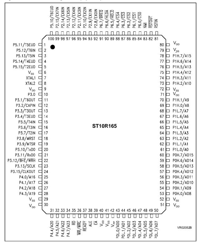
Figure 2. PQFP Pin Configuration (top view)
