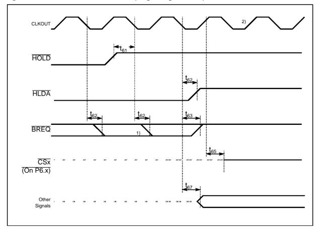
Figure 22. External Bus Arbitration, (Regaining the Bus)
