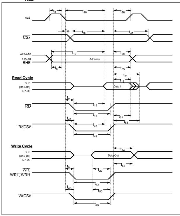
Figure 18. External Memory Cycle: Demultiplexed Bus, No Read/Write Delay, Normal ALE
