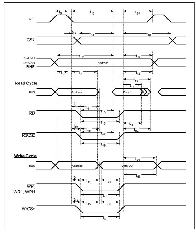
Figure 14. External Memory Cycle: Multiplexed Bus, No Read/Write Delay, Normal ALE
