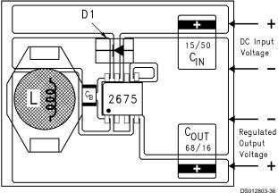
$C_{\text{IN}}$  - 15  $\mu\text{F},\,50\text{V},\,\text{Solid}$  Tantalum Sprague, "594D series"
