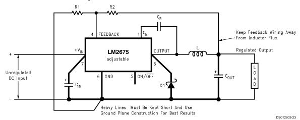
$C_{IN}$  - 22  $\mu\text{F},$  50V Tantalum, Sprague "199D Series"  $C_{OUT}$  - 47  $\mu\text{F},$  25V Tantalum, Sprague "595D Series"
