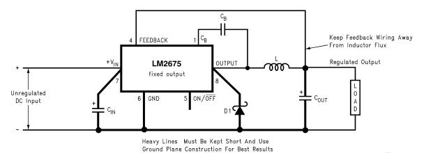
$C_{IN}$  - 22  $\mu F,$  50V Tantalum, Sprague "199D Series"  $C_{OUT}$  - 47  $\mu F,$  25V Tantalum, Sprague "595D Series" D1 - 3.3A, 50V Schottky Rectifier, IR 30WQ05F L1 - 68  $\mu H$  Sumida #RCR110D-680L
