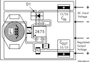
$C_{\text{IN}}$  - 15  $\mu\text{F},$  50V, Solid Tantalum Sprague, "594D series"
