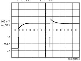
A: Output Voltage, 100 mV/div, AC-Coupled. B: Load Current: 200 mA to 1A Load Pulse
