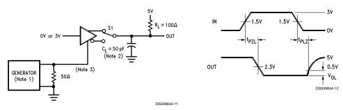
FIGURE 7. Driver Enable and Disable Times ( $t_{PZL},\,t_{PLZ}$ )
