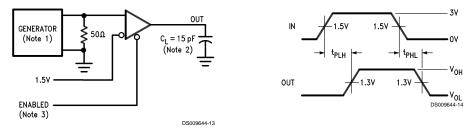
FIGURE 8. Receiver Propagation Delay Times
