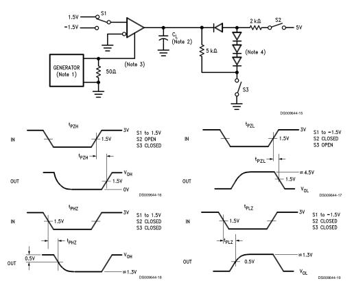
FIGURE 9. Receiver Enable and Disable Times
