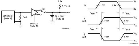
FIGURE 5. Drive Propagation Times
