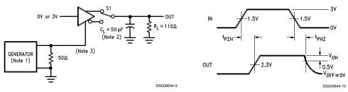
FIGURE 6. Driver Enable and Disable Times ( $t_{\rm PZH},\,t_{\rm PHZ}$ )
