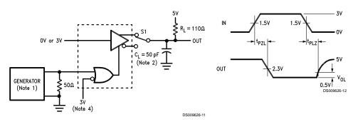
FIGURE 5.  $t_{\mbox{\scriptsize PZL}}$  and  $t_{\mbox{\scriptsize PLZ}}$
