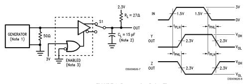
FIGURE 3. Propagation Delay Times
