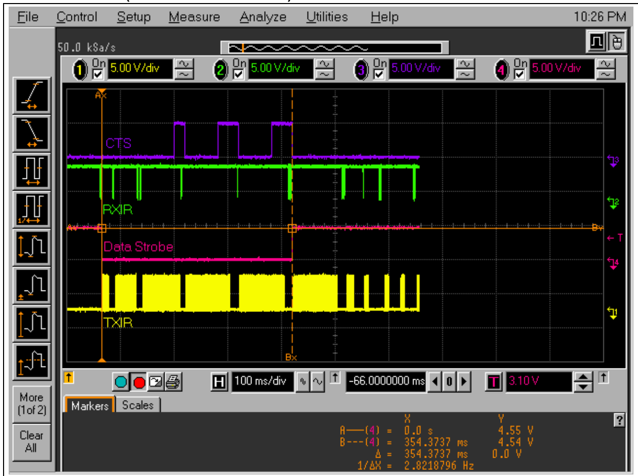
FIGURE 2-14: HOST CONTROLLER TRANSMISSION (S → P) OF A 250 BYTE PACKET (TO PC WITH IRDA PORT)
