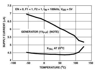
FIGURE 10. DISABLE SUPPLY CURRENT vs TEMPERATURE
