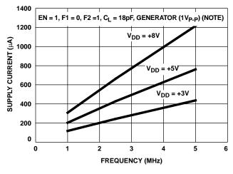
FIGURE 12. SUPPLY CURRENT vs FREQUENCY
