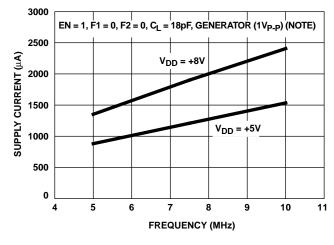
FIGURE 11. SUPPLY CURRENT vs FREQUENCY
