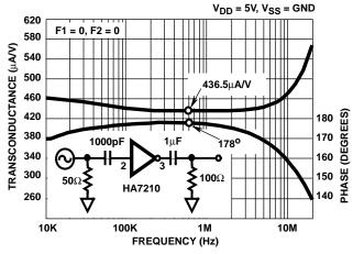
FIGURE 35. TRANSCONDUCTANCE vs FREQUENCY
