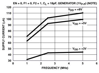
FIGURE 16. DISABLE SUPPLY CURRENT vs FREQUENCY
