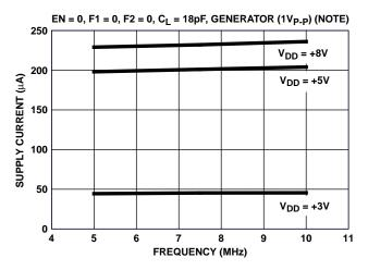
FIGURE 15. DISABLED SUPPLY CURRENT vs FREQUENCY
