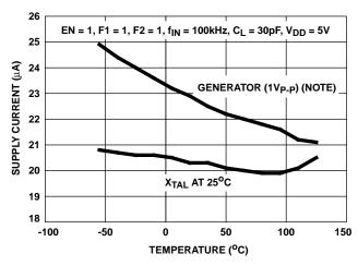
FIGURE 8. SUPPLY CURRENT vs TEMPERATURE
