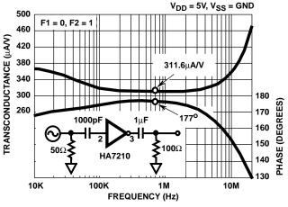
FIGURE 36. TRANSCONDUCTANCE vs FREQUENCY
