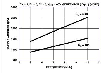
FIGURE 19. SUPPLY CURRENT vs FREQUENCY
