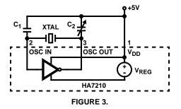
Typical values of the capacitors in Figure 2 are shown below. Some trial and error may be required before the best combination is determined. The values listed are total capacitance including parasitic or other sources. Remember that in the 10kHz to 100kHz frequency range setting the HA7210 switches in two internal 15pF capacitors.
