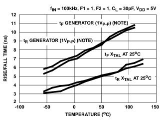
FIGURE 32. RISE/FALL TIME vs TEMPERATURE
