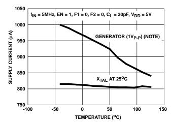
FIGURE 7. SUPPLY CURRENT vs TEMPERATURE
