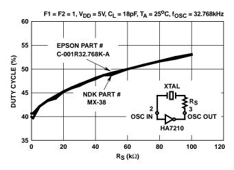
NOTE: Figure 39 (Duty Cycle vs R<sub>S</sub> at 32kHz) should only be used for 32kHz crystals. R<sub>S</sub> may be used at other frequencies to adjust Duty Cycle but experimentation will be required to find an appropriate value. The R<sub>S</sub> value will be proportional to the effective series resistance of the crystal being used.
