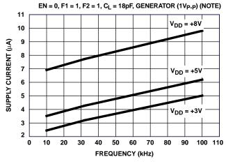
FIGURE 18. DISABLE SUPPLY CURRENT vs FREQUENCY
