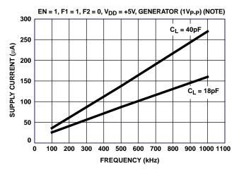
FIGURE 21. SUPPLY CURRENT vs FREQUENCY
