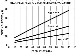
FIGURE 14. SUPPLY CURRENT vs FREQUENCY
