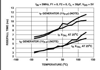
FIGURE 31. RISE/FALL TIME vs TEMPERATURE
