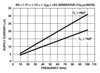
FIGURE 22. SUPPLY CURRENT vs FREQUENCY
