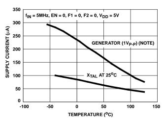
FIGURE 9. DISABLE SUPPLY CURRENT vs TEMPERATURE
