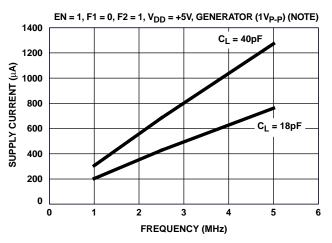
FIGURE 20. SUPPLY CURRENT vs FREQUENCY
