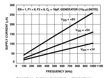
FIGURE 13. SUPPLY CURRENT vs FREQUENCY
