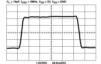
FIGURE 6. OUTPUT WAVEFORM ( $C_L = 18pF$ )
