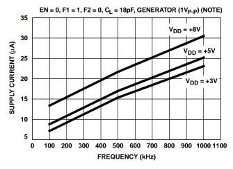
FIGURE 17. DISABLE SUPPLY CURRENT vs FREQUENCY
